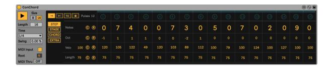
ConChord is not yet another step sequencer. Although it can be used as a simple 8 step sequencer, its features allow much more musical and complex patterns. Besides the classic note/velocity/length parameters (Step page), each step can have a variable pulse count to allow rests, pauses and repetitions (Stage page).
